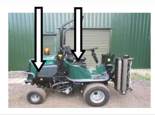
**Fixed cutting units:** Available in 8" and 10" options and offered with 4-8 bladed cylinders, fixed cutting units come fitted with a standard rear roller. Fixed cutting units are standard specification for cylinder ride on mowers and are better suited to flatter cutting surfaces.
