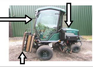
**Floating cutting units:** Available in 8" and 10" options and offered with 6-10 bladed cylinders, floating cutting units come fitted with both front and rear rollers to achieve a finer finish. Floating units are capable of cutting uneven surfaces and achieve a finer finish than their fixed head counterparts.
