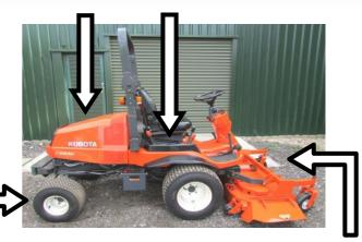
Side discharge rotary cutter deck: Most suited for dry grass cutting and therefore fairer weather conditions, side discharge decks require a more considered approach. Operator's should be mindful of cut discharge and ground speed to ensure an optimum cut.
