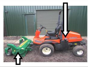
**Flail head:** Flail heads offer excellent versatility whilst maintaining impressive cut standards. Despite being better suited to tougher terrains than their belt driven rotary counterparts, flail heads remain capable of delivering a professional striped finish.
