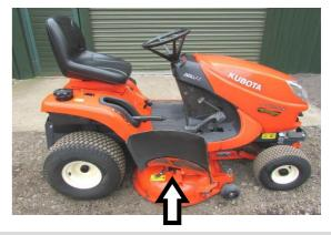
Side discharge [mulching] deck: Ride on mower mid-mount options include this versatile 42" PTO shaft driven cutter option. This is a 3 in 1 deck designed to cut, collect, and also mulch, depending on operator preference. 1/4" cutter height adjustment is also available at below seat level.
