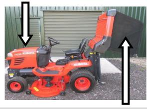
**Cut and drop or cut and collect:** Ride on mowers are available in either cut and drop or cut and collect specifications, the latter available with standard tip or high-tip collectors. Standard collectors are able to tip cut grass on a level whereas high-tip collectors offer more versatility.
